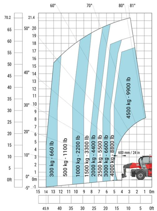
Machine on lowered stabilisers with 1500 kg jib with winch (Metric)
